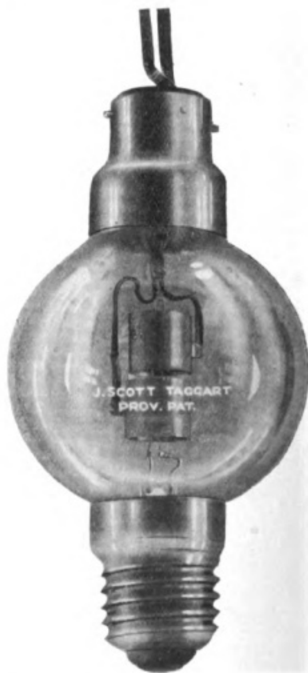
Fig. 3.—The Scott-Taggart-Ediswan Full-wave Rectifier (small power type).
